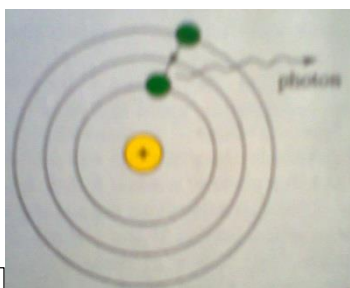
Fig: b An electron emits a photon when it moves to a lower energy level
